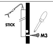
4. Fasten the transmitter and receiver by sticking them with the double-sided adhesive provided and the M3 screw. PROCEDURE TO FOLLOW FOR CASES OF MALFUNCTION OR BREAKDOWN Please note that the back of the receiver is fitted with a red LED, whereby operation of the barrier can be checked:
