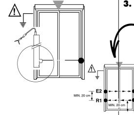
3. Insert the heads and the cables in the profiles.
